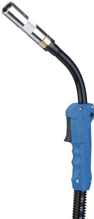
MIG TORCH--QTC500A Welding Gun QTC TYPE Rating:500A CO 2 420A mixed gas, 60% duty cycle. wires:1.2-1.6mm
