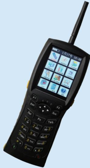
The water meter handheld device communicates with water meters wirelessly, mainly used for wireless water meter data reading/writing, parameter setting, production testing, and installation & debugging. Equipped with a built-in rechargeable battery, it requires no external power supply and features long communication distance, simple operation, easy portability, and high cost-effectiveness.
