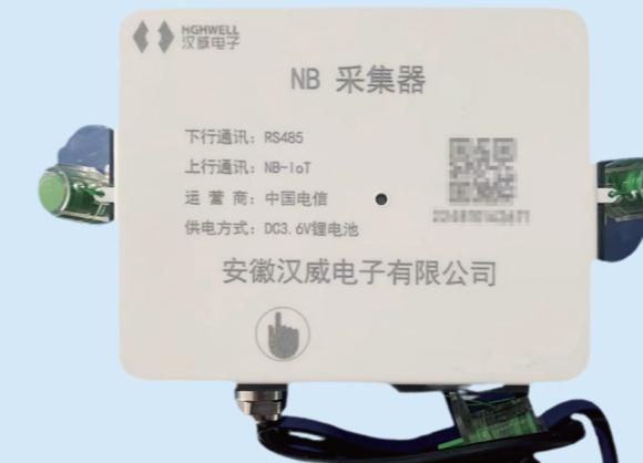
It adopts NB-IoT communication technology, featuring low power consumption, long service life with battery power supply, wide coverage, strong network compatibility and full-network support. It has functions of timed data collection and active data reporting, and its flexible configuration can meet various needs, making it suitable for all types of scenarios.
