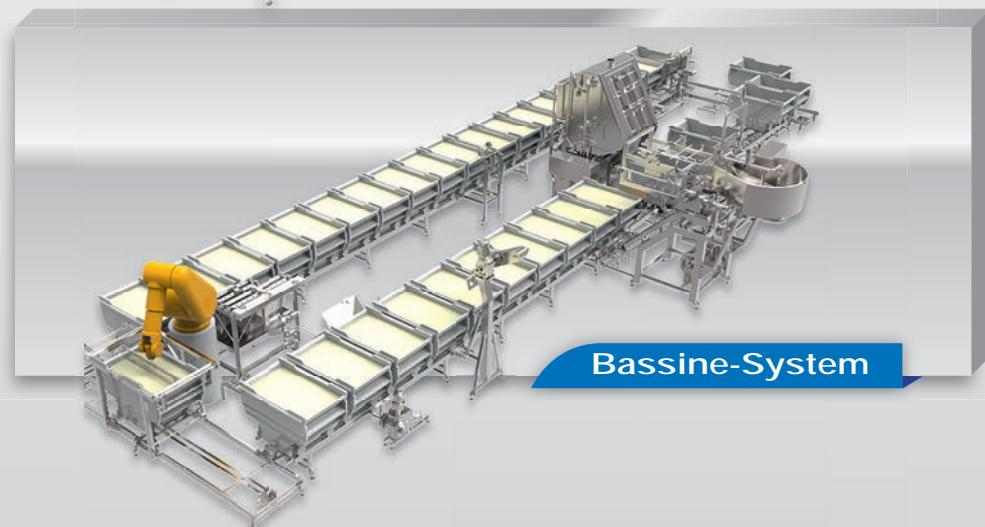
Curd preparation in Bassines moving over a conveyor system.
