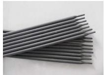
**Uses:** Used for welding key medium-carbon steel and low-alloy steel structures (under pressure and moving loads), such as 16Mn, 09Mn2Si, 09Mn2V and A, B, D and E steel for ships, etc., and also used for welding on thick plates and hard-to-weld carbon steel structures.
