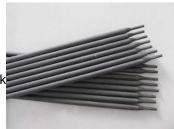
Uses: Used for welding corrosion-resistant 0Cr19Ni9 and 0Cr19Ni11Ti stainless steel structures below 300 ℃.
