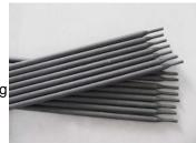
**Uses:** Used for welding 0Cr18Ni12Mo2 stainless steel equipment working in organic acid and mineral acid (non-oxidizing acid) medium, and also used for welding dissimilar steel.
